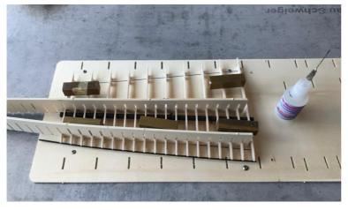
At the end we check again the correct alignment of all ribs and glue all whole ribs (not the half-ribs) to the tube. Tip: for correct alignment we use weights to fix the wing part neatly.
