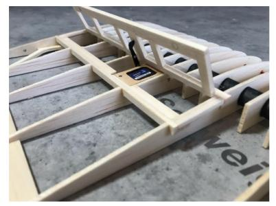
Should our solution be used for the flap opening, a servo arm extension is required. For the servo arms we recommend our GFK extension, which is available as an accessory together with the matching servo frames.. We also have a video for the functional mode:
