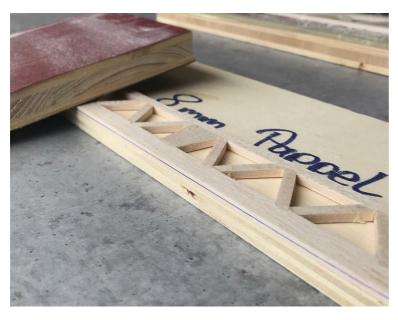
As you can see in the picture, we put the rudder on an 8mm thick plywood. When sanding the rudder with a sanding board, make sure that the sanding board rests on the trailing edge of the tail unit and the edge of the table. So we grind the trailing edge to a point from both sides (approx. 1mm) up to our auxiliary line. In contrast to the trailing edge, which we have just sharpened to a point, we are grinding the leading edge of the tail units round.
