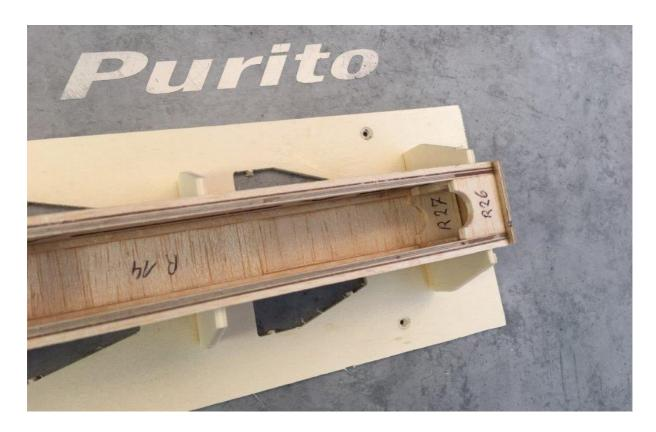
Now parts R25 are glued to both sides of the fuselage, part R26 should be glued to the bottom of the fuselage and part R27 to the top of the fuselage, centered between the two parts R25 (see picture). The parts R25-R27 are there to fit the fuselage to the spinner later.
