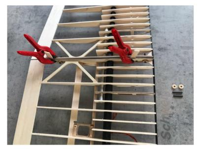
To prevent twisting of the wing ears on the center section, the accessory package includes dowel pins with a diameter of 2.5mm made of CFK.
