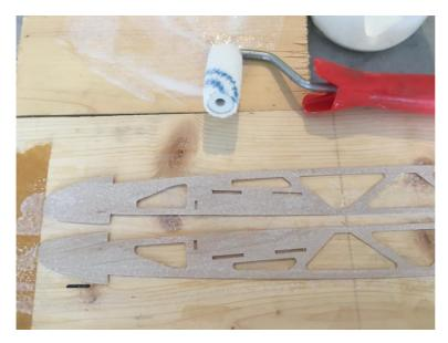
As shown in Fig. 3, we use a roller for gluing R9 and R10. This allows the glue to be applied in an evenly thin layer. Press the parts together for several hours.
