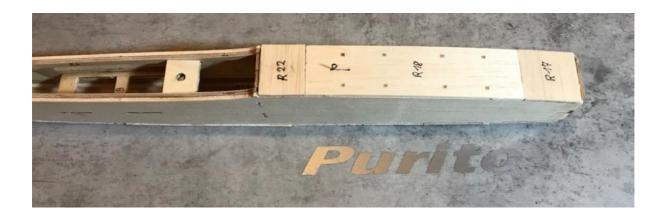
The plywood part R23 is glued inside the canopy to the fuselage tip center, serving as a tongue. Glue the balsa part R21 to the end of the canopy between the plywood strips. Bend a steel wire into L-shape and glue it together into a Bowden cable into the inside of the canopy as a fastener.
