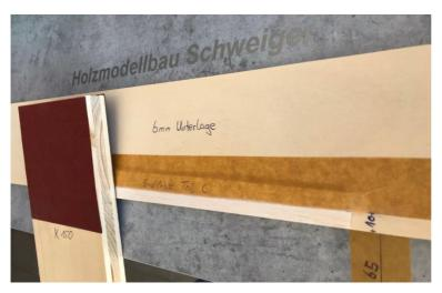
The end strips are ground before installation. To do this, place the first and last ribs on the end strip and mark the end of the ribs on it.
