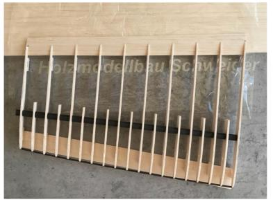
For the end strips (sash part A,B,C), sanding is performed on a base of 6mm at a distance of 60-65mm from the edge of the table. This distance is the same for all end strips of the wing.
