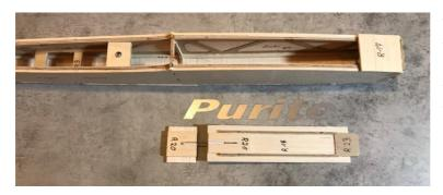
Then glue part R20 centrally on the fuselage planking R22 and fit it together with the canopy in the canopy opening in the fuselage.
