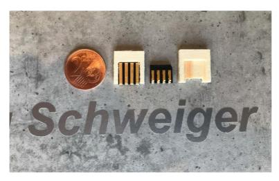
We use a 5-pin spring contact for the power connection to the fuselage. This is also available from us as an accessory. As you can see in the picture, these accessories also include milled plywood parts that fit the spring contact accurately into the wing mount.
