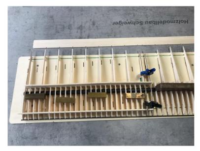
After that, the two plywood pieces A1V (for the surface screw connection) can be placed. These belong in the recess of the plywood ribs A1. The top side is marked by the recess for the screw head.
