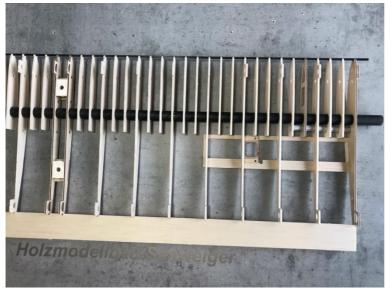
The component A2V is located on the 8mm balsa board and is glued under the plywood part A1V and pierced flush. Tip: insert a drill with a diameter of 5mm through the balsa blocks A2V when gluing so that the holes are exactly on top of each other.
