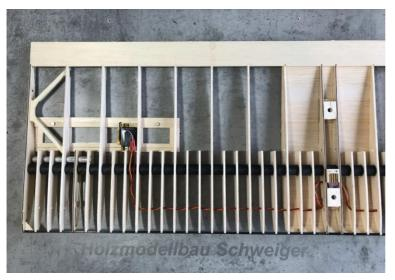
provided for them in the airbrake. The flap is inserted into the wing. The magnets can now be placed on the underside of the KF3 component. The magnets now align themselves. This means that the remaining magnets from the underside of the wing can also be glued. The magnetic attraction force is thus already sufficient in this version. If a higher attraction force is required, the magnets can be embedded a little deeper.
